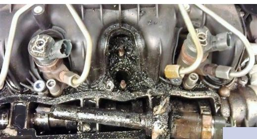
To solve this fault, it is necessary at least to remove the injectors and **change the washer** and gaskets that are installed in this area, as well as the nuts and studs that hold the injectors.
